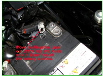
Remove the Negative (ground) Terminal first. Then remove the Positive Terminal and attach the RED terminal connector and reattach the Positive Terminal. Finally attach the Negative connector and reconnect the Negative Terminal. Removing the Negative first and reconnecting it last eliminates the possibility of shorting the Positive.
