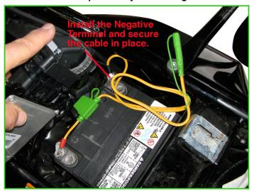
Securily fasten both terminals and route the cable so that the seat or other parts don't pinch the wires. The in-line fuse protects the wire should it become shorted but do take the time to prevent any chaffing or crushed wires from oddcuring when reassembly id done.
