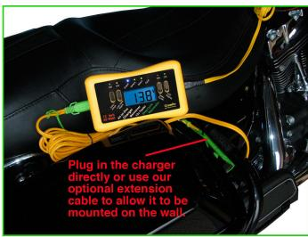
After the cable is routed to a location that will be easy to reach, use the two loops that are on the green connector to tie down the cable. The loops provide an easy attachment point for the cable end. Plug the cable into the charger or the optional extension cable and the charger will do the rest.
